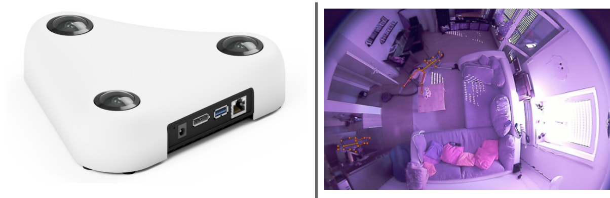
Figure 1.1: Left: HemiStereo Sensor developed by the cooperation partner 3DVisionLabs is shipped with NVIDIA 's AI embedded processor Jetson TX2 . The sensor is mounted on the ceiling and is able to process all data on the device itself. Right: An image captured by the sensor and processed by the inferics pose estimator.
