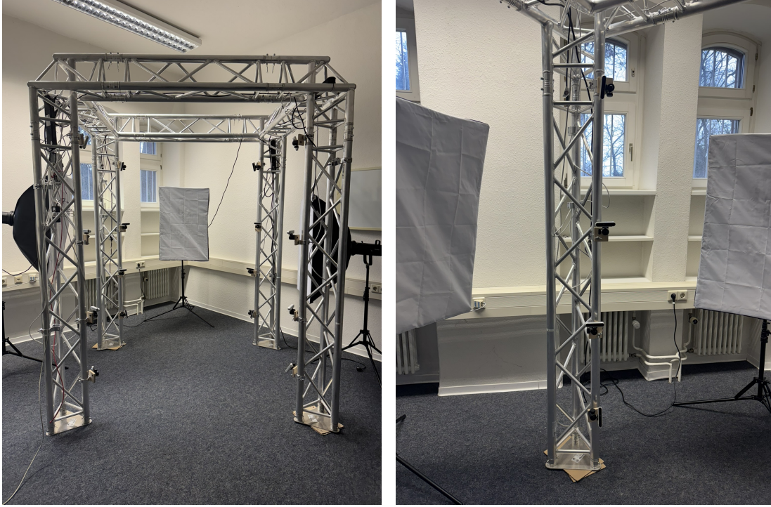
Figure 4.2: Multi-camera setup consisting of 16 RealSense D415 cameras. The top and bottom cameras are mounted vertically, while the remaining cameras are positioned horizontally.
