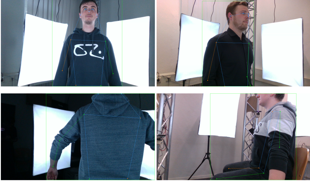
Figure 5.2: Scanner images with detection results showing hip keypoint errors. Partial truncation leads to incorrect predictions, as the model is uncertain whether the hips lie inside or outside the visible region.
