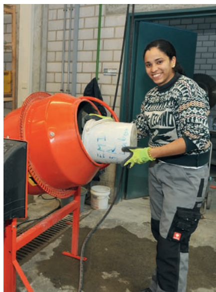
Preparing Concrete Samples
