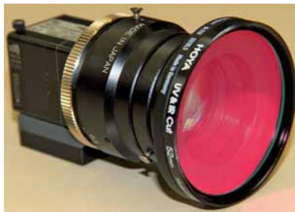
Fig. 1: Plenoptic camera from Raytrix GmbH (Model R5)
