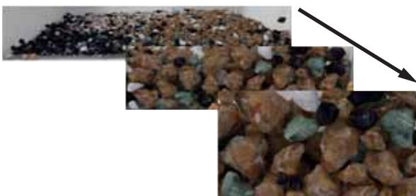
Fig. 5: Packing of grains in a computational domain using grain topology from Figure 4 and a sedimentation rule specified for the underground around the drilled well in Spain
