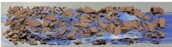
Fig. 6: Flow streamlines through the porous grain structure
