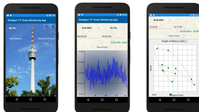
Fig.1: The main page, position-time series and graph of tower motion visualisations of the app
