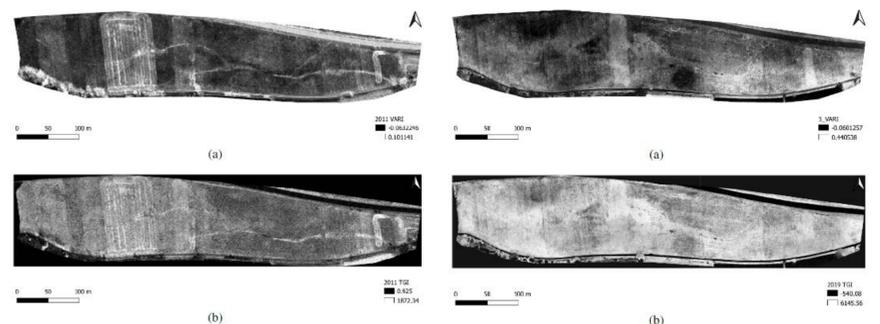
Figure 3. Aerial (left) and UAV (right) multispectral image analysis in ditch mapping.
